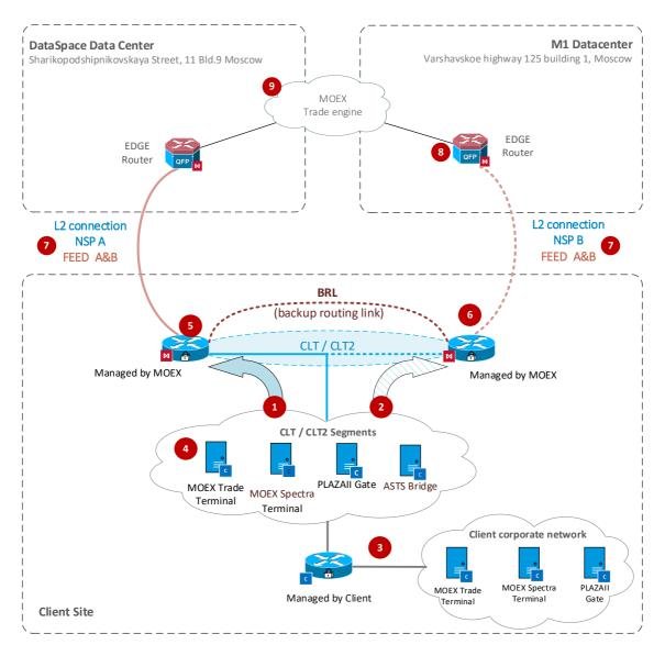
**CLT segment** is a dedicated segment of the Client's network designed to install specialized software and exchange systems (item 4) as well as establish a L3 link to the Client's internal network (item 3). VLAN (IEEE 802.1Q standard) is supported; VLAN ID must be transferred to MOEX's specialists at the setup stage.
